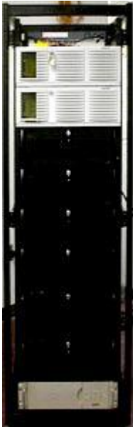
Figure 4. The ImageLinks Beowulf cluster consists of 12 nodes, RAID disk drives, 100BT Ethernet Switch and power conditioning.
