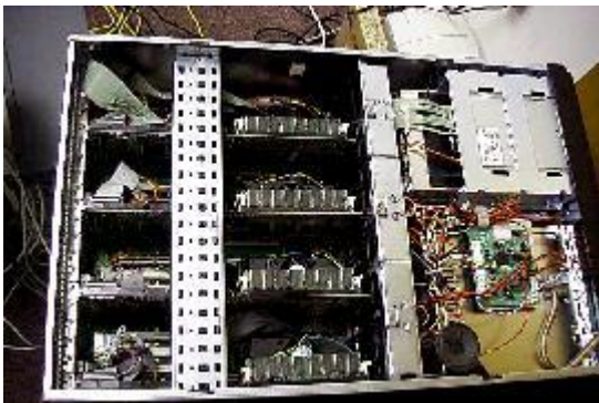
Figure 5. Four 650MHz Pentium III nodes with 384 Meg of memory in a 4U rack mounted unit.
