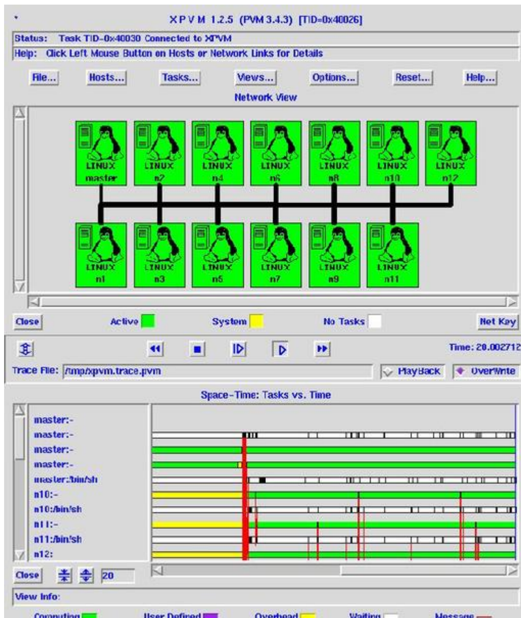
Figure 1. Screen shot of the bWatch program of the ImageLinks Cluster. The red lines indicate communication between nodes and demonstrate that the process is CPU-bound.
