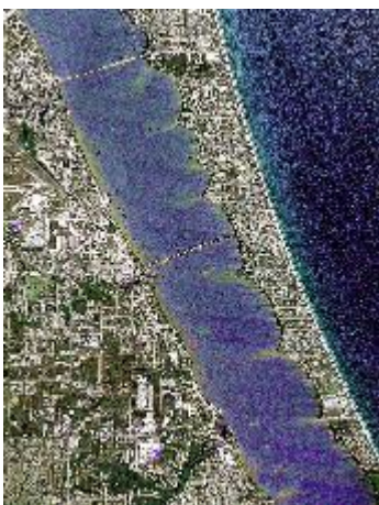
Figure 2. A section of a fused satellite image of Melbourne, Florida. This image was formed with the color from Landsat 5 combined with the 5m spatial resolution of the Indian IRS 1C satellite.
